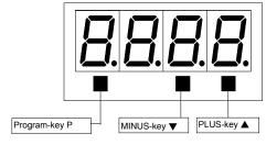
The basic adjustments concerning to the following program example are the ground parameters after a total reset occurring through a power on with pressing **P**-key (see previous page).
